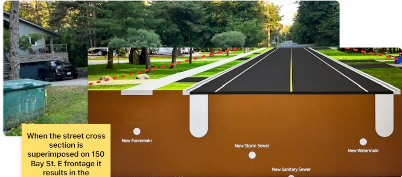
When the street cross section is superimposed on 150 Bay St. E frontage it results in the elimination of >50% of current driveway and off street parking.
