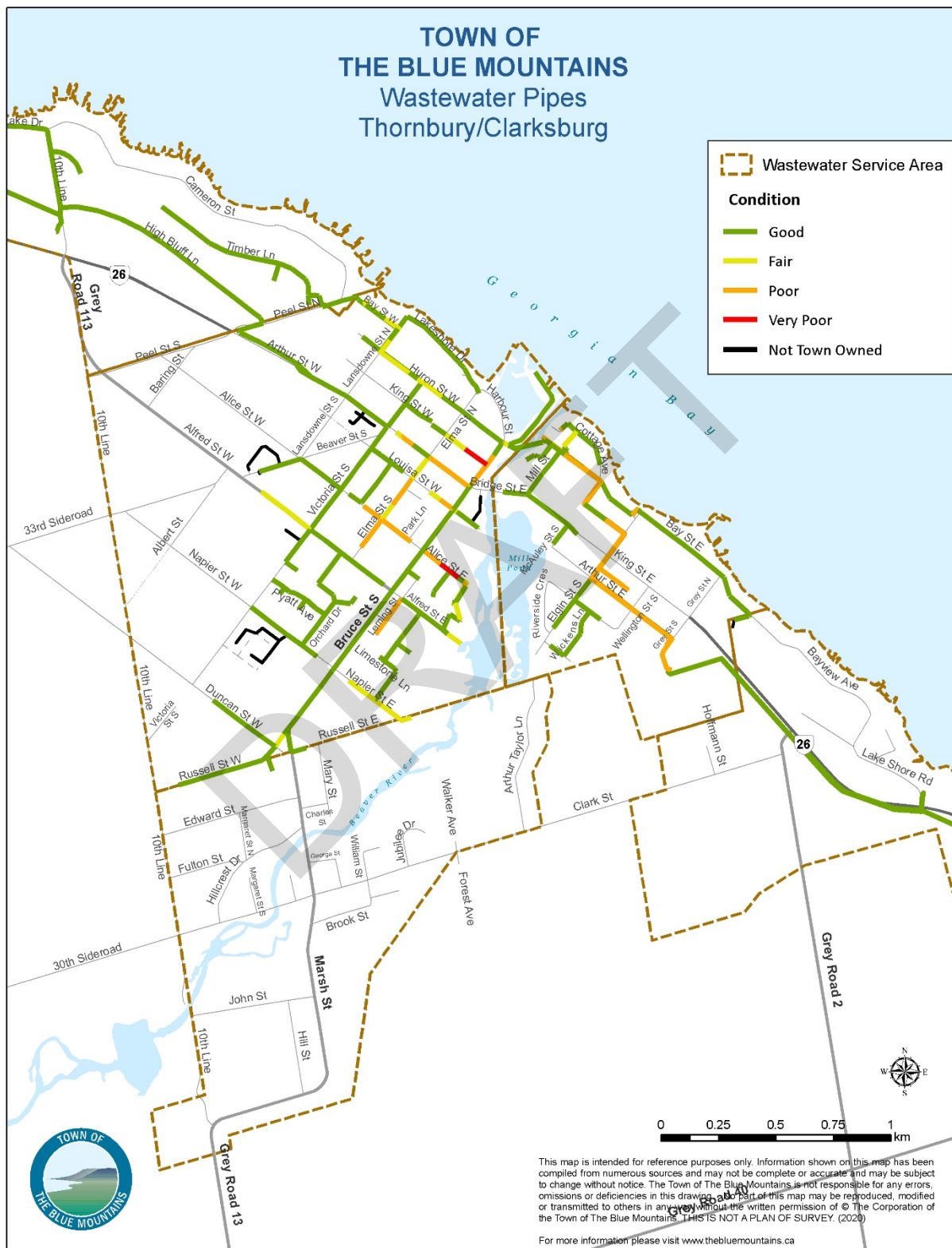
Map 2 Town of The Blue Mountains Wastewater Pipe by Condition Rating-Thornbury/Clarksburg
