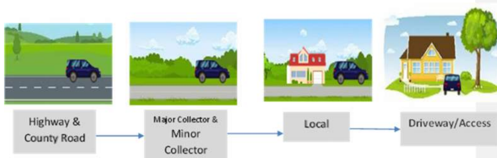
Figure 8-1: Road Classification Hierarchy for TBM
