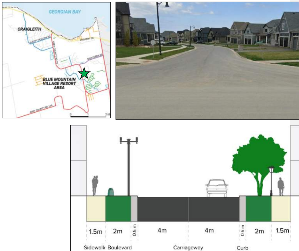
Figure 8-11: Proposed Cross-Section Treatment for Local Roads
