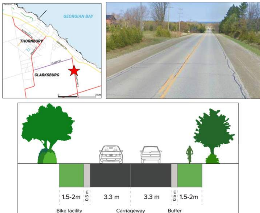
Figure 8-7: Potential Cross-Section Treatment for County Rd 2
