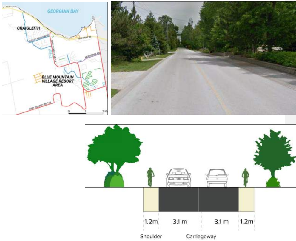
Figure 8-10: Proposed Cross-Section Treatment for Sleepy Hollow Road
