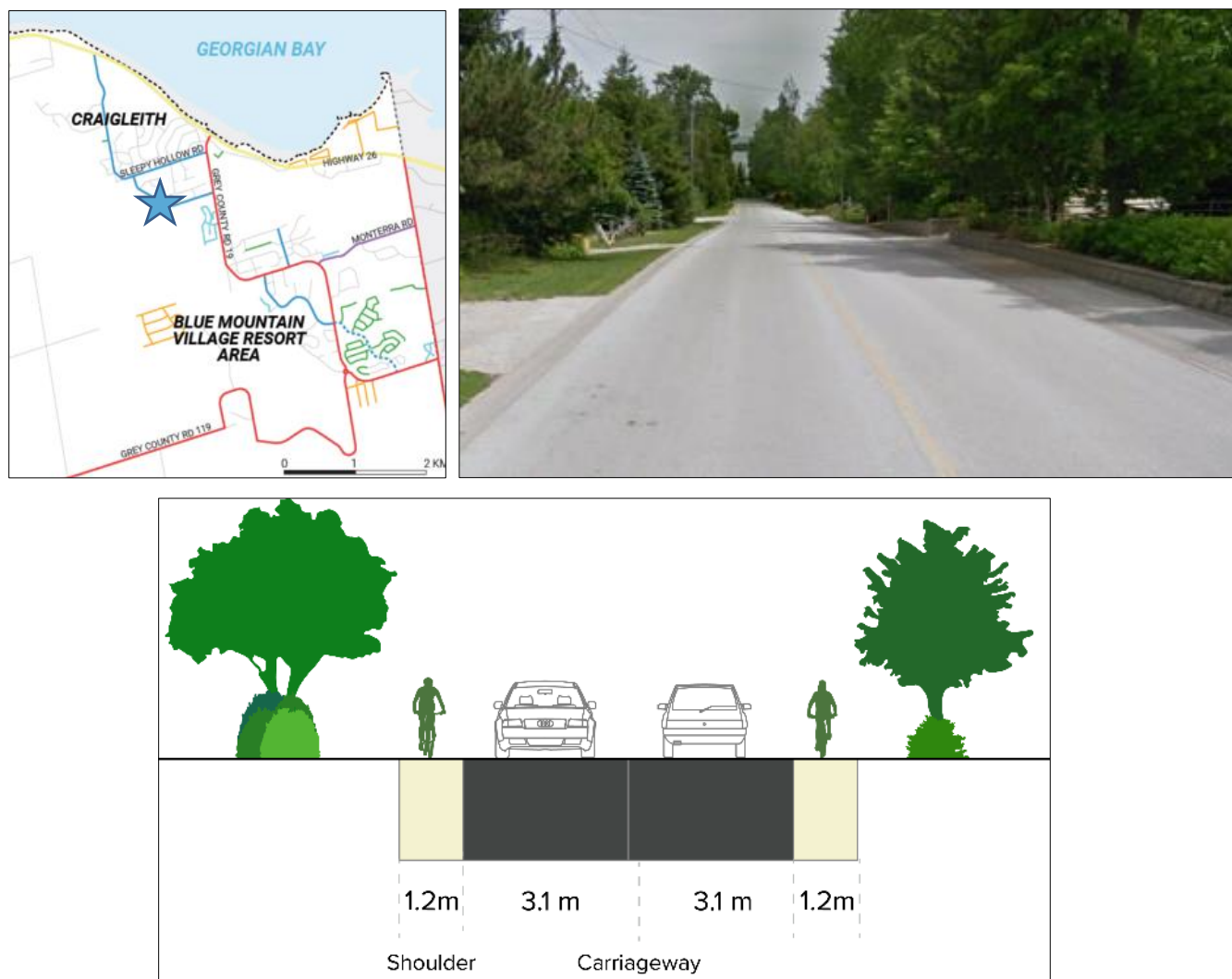
Figure 8-10: Proposed Cross-Section Treatment for Sleepy Hollow Road
