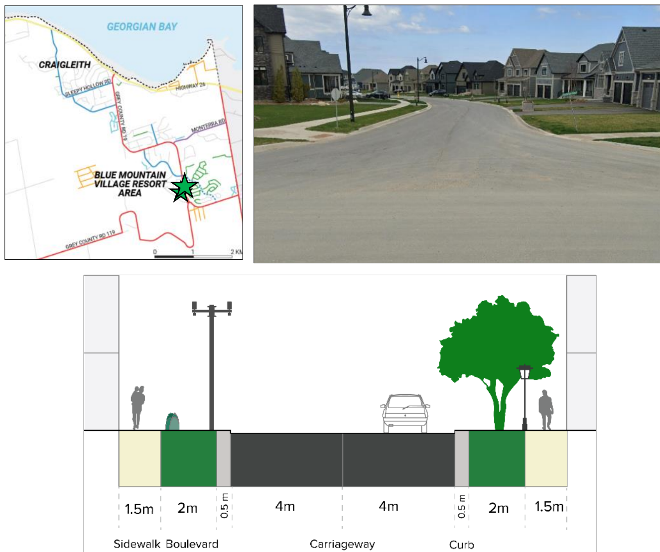
Figure 8-11: Proposed Cross-Section Treatment for Local Roads
