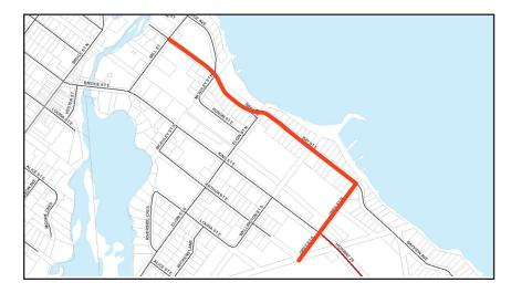
The Town of The Blue Mountains needs to install a secondary sanitary forcemain from the Mill Street Pumping Station to the Thornbury Wastewater Treatment Plant (TWWTP) to service growth in the west portion of the municipality. The secondary forcemain will begin at the Mill Street Sewage Pumping Station and follow Bay Street East to Grey Street, and then proceed south on Grey Street to the treatment plant.
